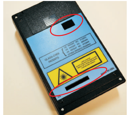
Above: Back of GC3001 meter with the two lenses circled. Use clean compressed air to clean the lenses.
